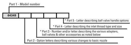
\* Parts 3 and 4 not applicable for D-1, D-2 or D-3 configurations
