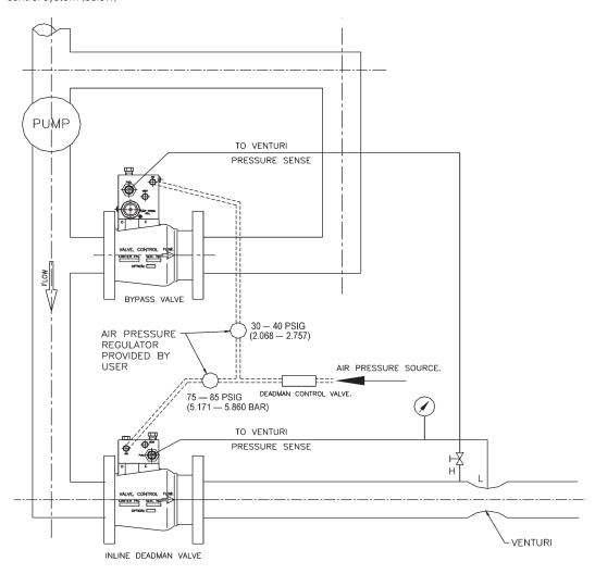
Note: The inline and bypass valves shall be installed in such a way that the pressure sense ports shall be located in the top position of both valves to achieve satisfactory bleeding of trapped air
